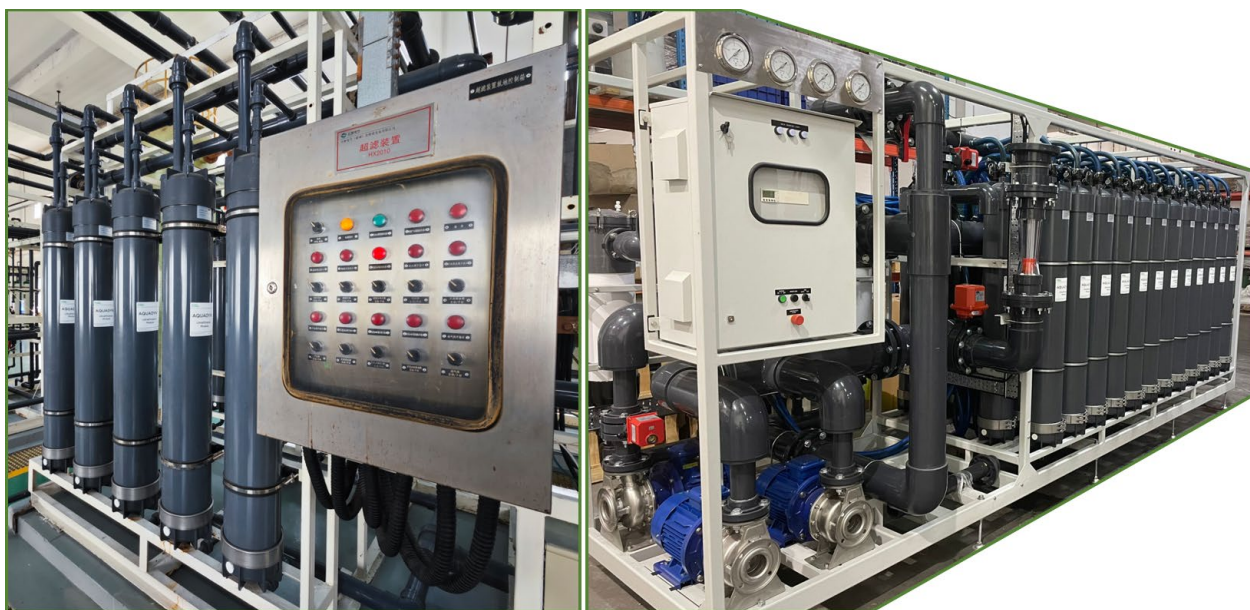
Figure 6. Rack with AQUADYN® UA860-HP UF modules
